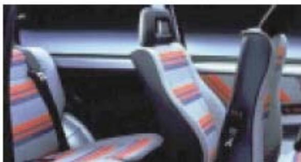
In the last five years the density of polyurethane for major applications has been reduced by 30 to 40 per cent while still maintaining the same mechanical properties. Seating foam, for instance, has one of the lowest densities of any plastic material used in a car: 0.03 to 0.05 g/cm<sup>3</sup>. Polyurethane foam in headliners is another good example with a density of 0.02 to 0.04 g/cm<sup>3</sup>.
