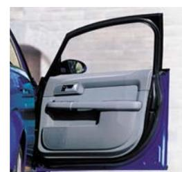
and PU as the binder has exceptionally high mechanical strength. Wall thicknesses of only 1.5 to 2.0 mm can be achieved. The weights of the end products are also extremely low at 1,250 to 1,600 g/m<sup>2</sup>. Weight reductions of up to 2.5 kg per vehicle can be achieved in comparison with traditional materials. The use of large proportions of renewable raw materials further reduces the CO<sub>2</sub> in-balance.
